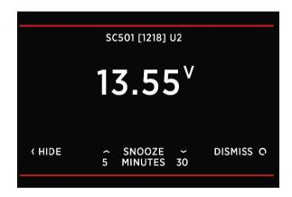
If at least one alarm is active, then an alarm entry on top in the menu settings is displayed. From there you can view all currently active alarms.
