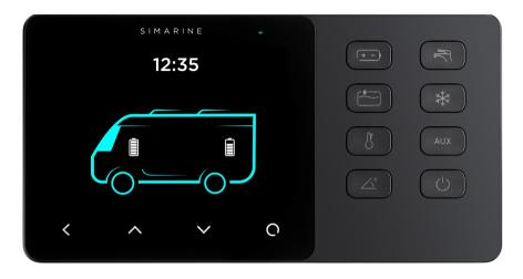
After the first power-on, there are no batteries and tanks displayed. Long press the 🖸 button to enter the settings menu.
